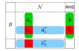
Assume  $\widehat{m{b}} \geq m{0}$  Seek  $\widehat{m{c}}_{\scriptscriptstyle N} \geq m{0}$ Scan  $\widehat{c}_{j} < 0$  for q to leave  $\mathcal{N}$ Scan  $\widehat{b}_{i}/\widehat{a}_{iq} < 0$  for p to leave  $\mathcal{B}$
