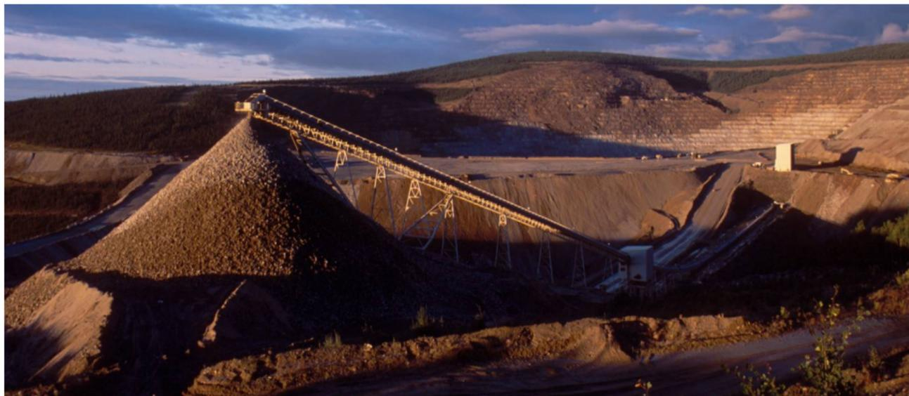
▶ stockpile allows to store mined material before processing
