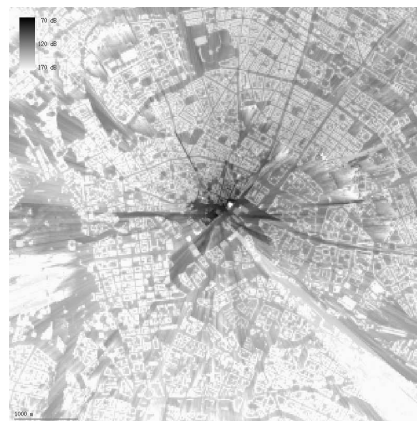
(d) Berlin, e-plus predictor with 100 m resolution height, clutter, vectorized street and building data
